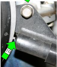
terminals) to hold the timing at (what the ECU thinks is) 10°. Skipping this jumper will allow the timing to vary and won't give you an accurate reading. Turn as many loads off as possible (HVAC fan, lights, radio, etc.) and be sure the car is warmed up but the fans aren't running while you check the timing.
